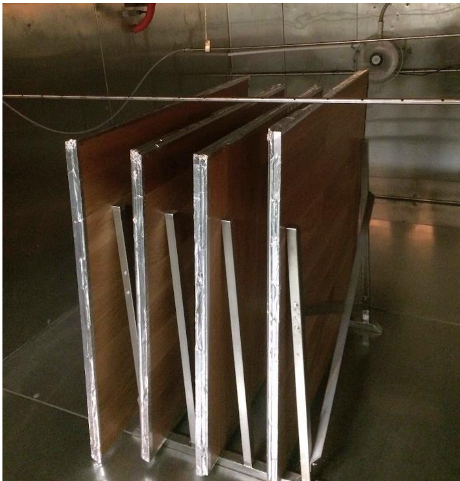
Figure 1. Specimens mounted on a back to back configuration in large chamber CONTRACT NUMBER 301013685 10.1
